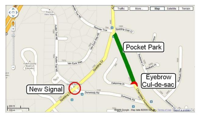
Minor adjustments may need to be made to the intersection of Dunwoody Road and Chamblee-Dunwoody Road, particularly with pavement markings to redirect the primary flow of traffic. Alternately, minor alignment changes could be made to bring the former main street into more of a side-street configuration.
