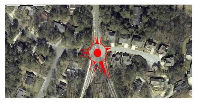
Another construction option for this intersection is a roundabout. The right of way requirements would likely have a similar impact as the left turn lane solutions and would provide a better level of service and good safety performance.
