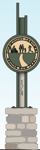
1 DISTANCE MARKER (WITH AND WITHOUT STONE BASE) - FRONT ELEVATION SCALE: 1/2" = 1'-0"
