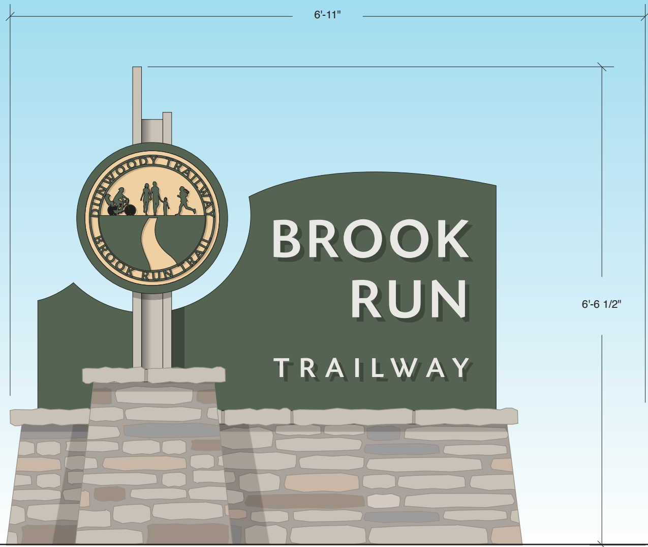
1 TRAILHEAD MARKER - FRONT ELEVATION SCALE: 3/4" = 1'-0"
