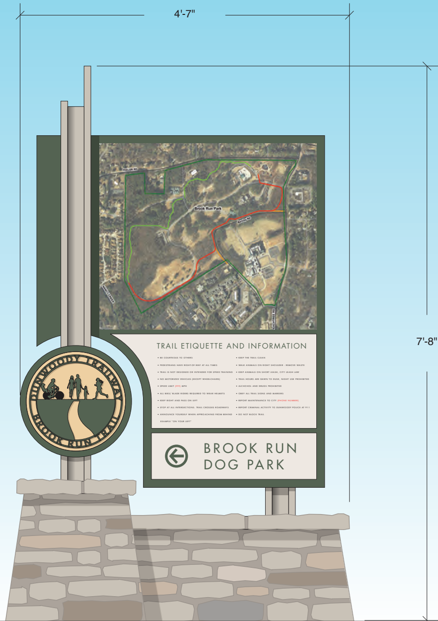
1 TRAIL MAP KIOSK - FRONT ELEVATION SCALE: 3/4" = 1'-0"
