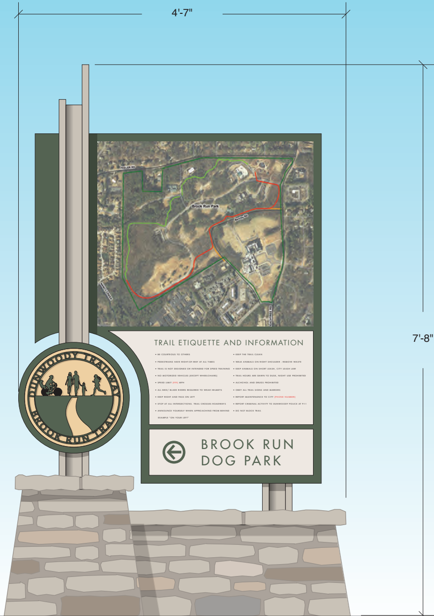
1 TRAIL MAP KIOSK - FRONT ELEVATION SCALE: 3/4" = 1'-0"
