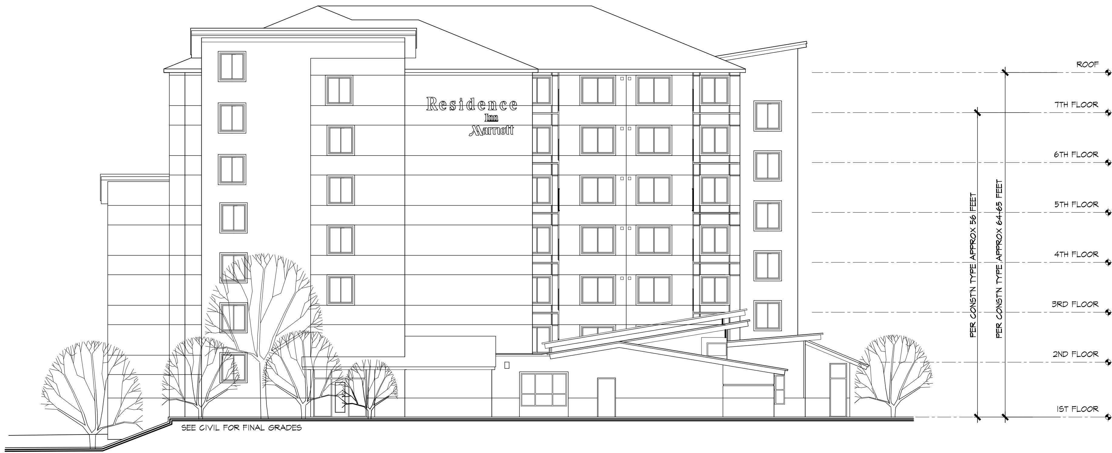
2 STREET ELEVATION (FACING NORTH) SCALE : 3/32" = 1'-0"
