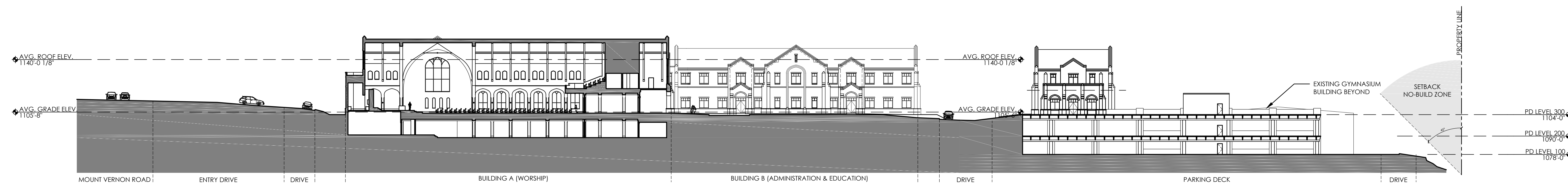
M01 ARCHITECTURAL NORTH-SOUTH SITE SECTION A501 1/32" = 1'-0"
