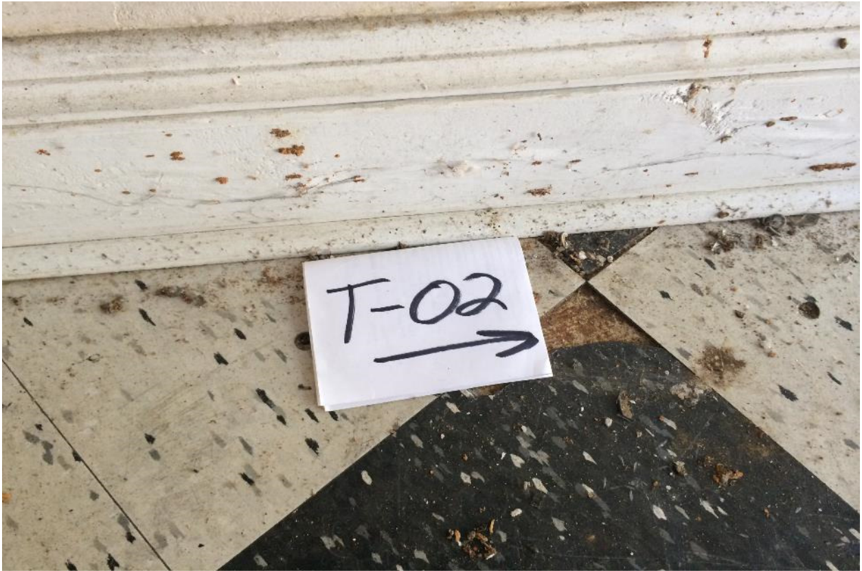
Plate 53: Laboratory analyses did not detect asbestos minerals within the black floor tile from sample TS-02 but did detect 5% chrysotile asbestos in the mastic from sample TS-02 collected from the Theatre Building lobby area.
