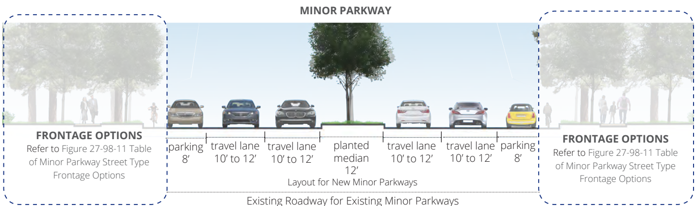
Figure 27-98-10 Minor Parkway Street Section - Existing and New
