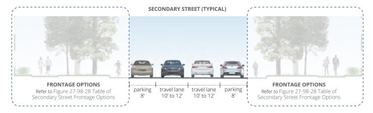
Figure 27-98-26 Secondary Street Type Section - Typical
