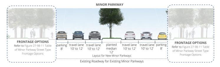
Figure 27-98-10 MInor Parkway Street Section - Existing and New
