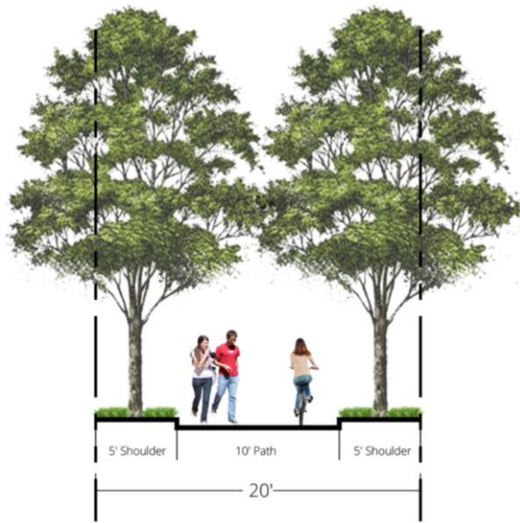
Figure 27-107C-5 New Pedestrian Path (not to scale)
