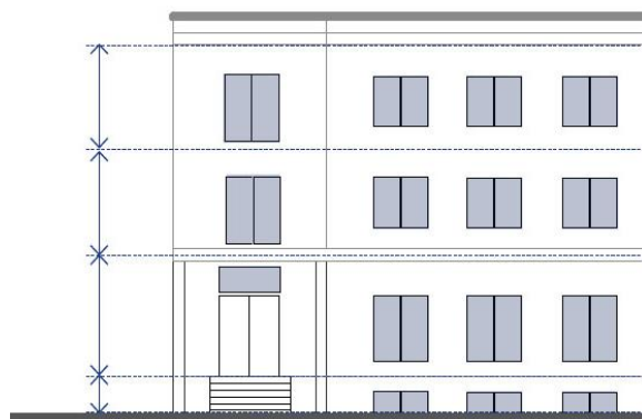
Figure 27-107D-4 Measuring Fenestration per Façade
