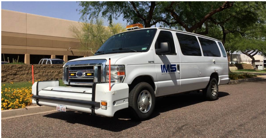
Figure 5 – Laser Road Surface Tester (Laser RST)
