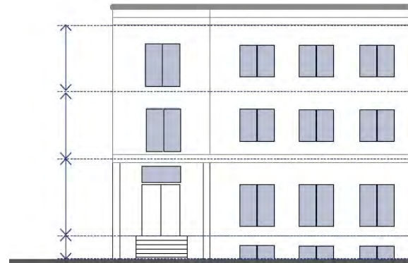
Figure 27-107D-4 Measuring Fenestration per Façade
