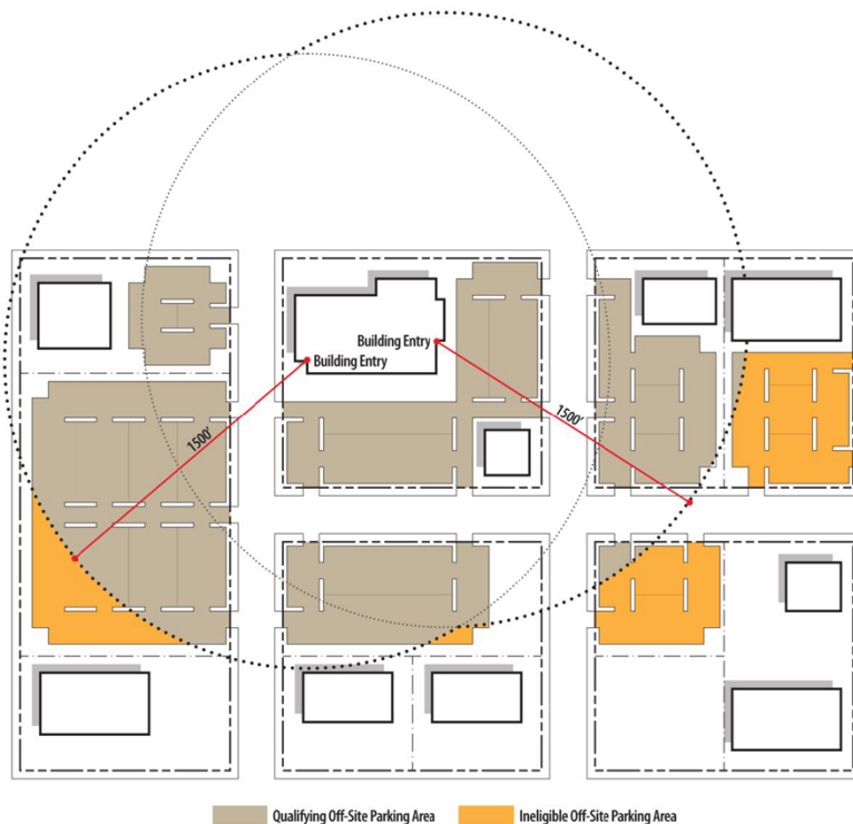
Figure 12-1: Off-site Parking, Maximum Distance Measurement
