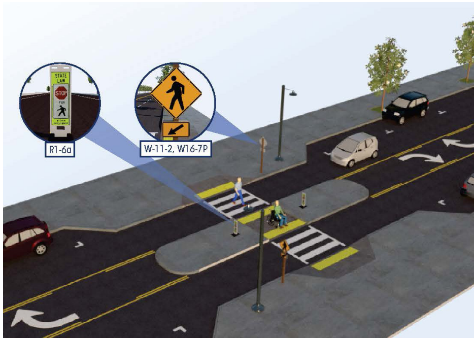
A combination of long crossing distances and multiple lanes of oncoming traffic warrants the installation of a pedestrian refuge island.
