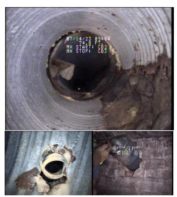
Corrosion with visible holes Multiple private drain tie-ins
