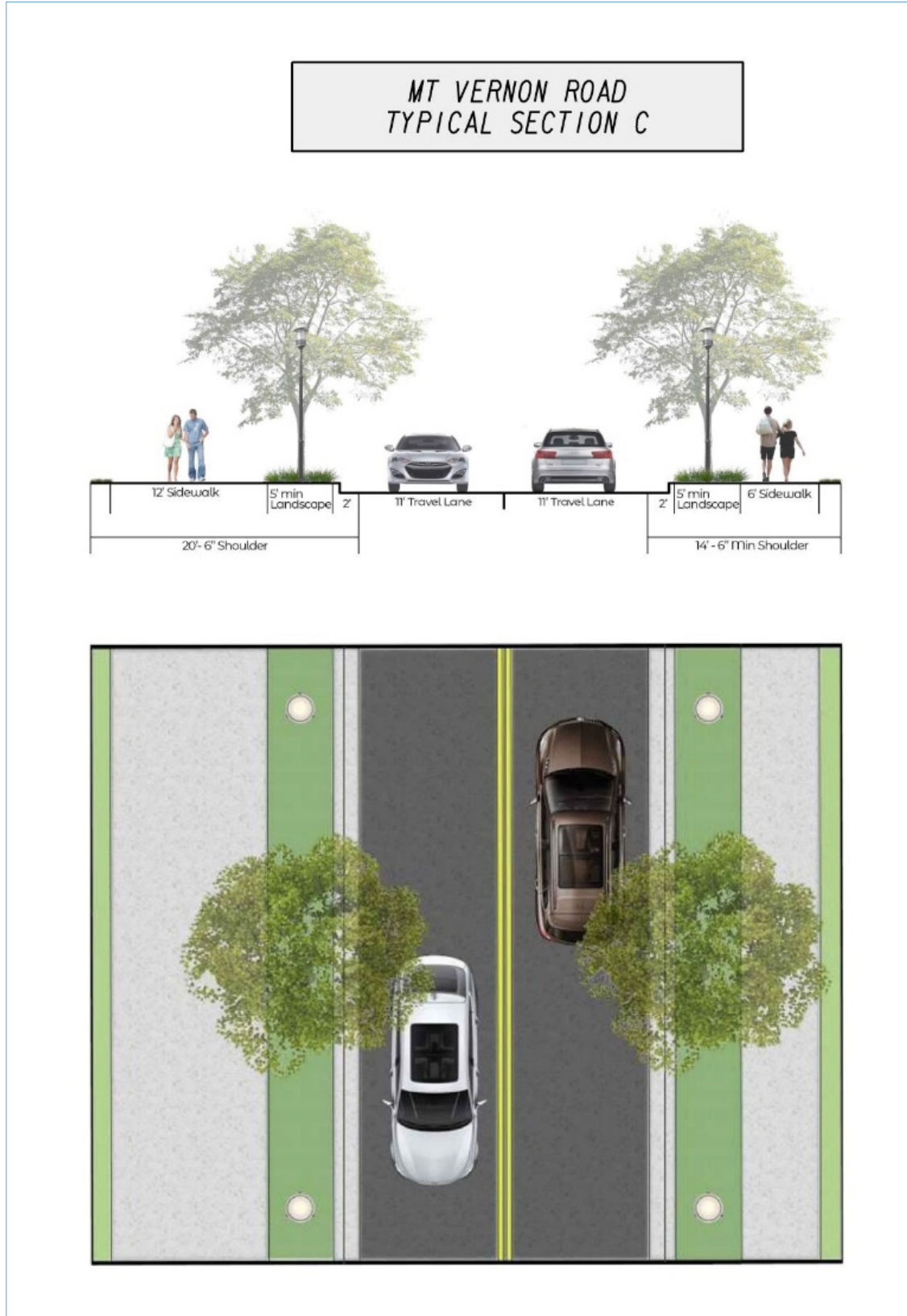
Figure 14-6: Mt Vernon Road, Typical Section C
