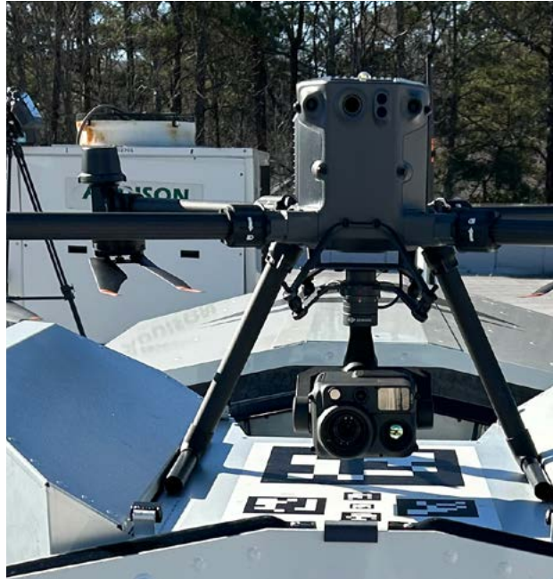
DPD's Aerodome drone pod installed on top of City Hall
